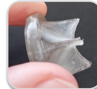
Injection molding (heart valve)
