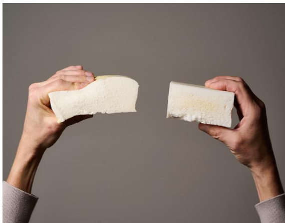
r.T. CO 2 -self-blown NIPU foams
