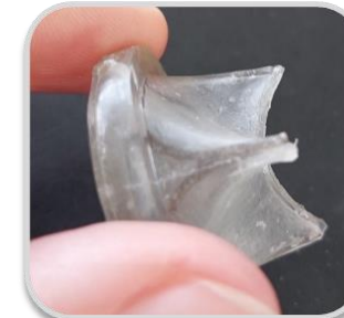
Injection molding (heart valve)
